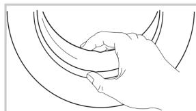
Wipe the glass and seal after each wash to remove lint and stains. If lint builds up it can cause leaks.
