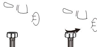
2 Connect the other end of inlet pipe to the inlet valve at the backside of product and fasten the pipe tightly clockwise.
