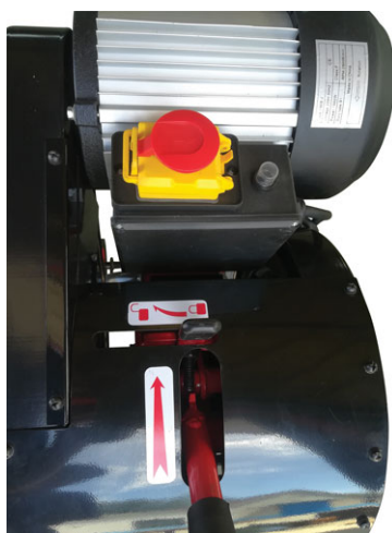
Close-up image of lever and emergency stop.
