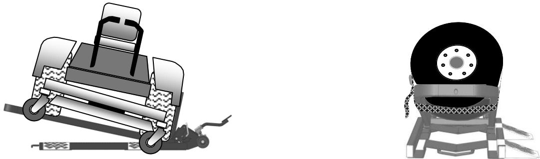
5– Lift completely until the safety stops lock.
