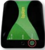
The status indicator is the outermost light on the side of the EquiAlarm. The status indicator is a special light that can light up in 3 different colours: blue, green and red. You can read the status of the EquiAlarm via the status indicator flash sequence. For example, if the light is flashing Green, the EquiAlarm is OK. On the contrary, when the status indicator is flashing red, the battery needs replacing.
