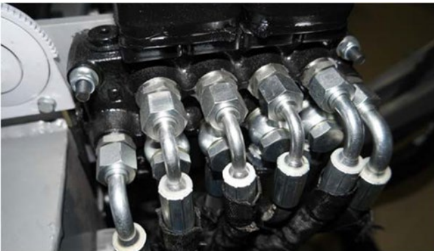
Fig. 54: Control block on right side in direction of travel.
