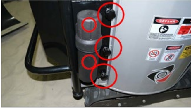
Fig. 43: Remove the container and loosen the screws on the right.
