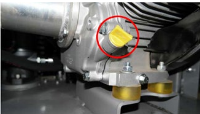
Fig. 6: Close up of the oil plug/dipstick.
