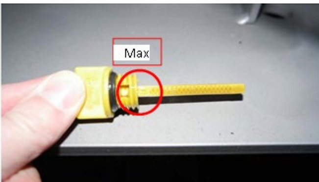
Fig. 7: Dipstick with max. mark.
