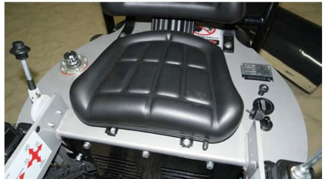
Fig. 24: Seat with in-built switch.
