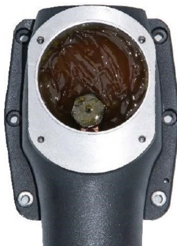
Example of new lubricant (before use)
