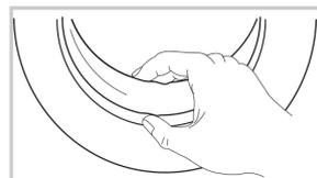
Wipe the glass and seal after each wash to remove lint and stains. If lint builds up it can cause leaks.
