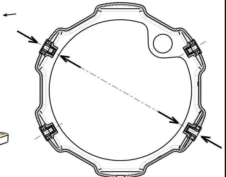
**MONTAGE SUR BUSE BETON - MONTING ON CONCRETE STAND
