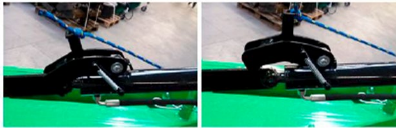
Figure 14 Locking the cylinder: A) locked, B) open
