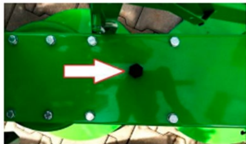
Figure A – oil fill plug
