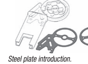
Automatic alum die-casting hinge with an inner steel plate strengthening.
