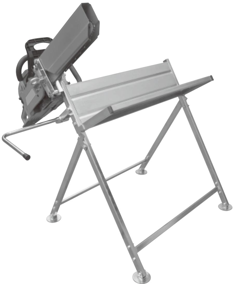
Fig 3. Carefully lower the chainsaw bar into position between the two solid blocks in the pivot clamp and ensure a 2 cm gap between the body of the chainsaw and the clamp. Make sure that the bar is approximately 90 degrees to the clamp and well clear of the chain before tightening the bolt. Once tightened, test the arc of travel to make sure that the chain bar does not touch any part of the sawbench.
