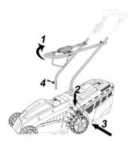
Attach the cable with the two cable clamps.
