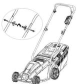
■ Insert the lower handle into the slot(2).
