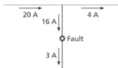
3. A fault is indicated by a drop in current flow between two checkpoints. The fault will be somewhere between the two checkpoints.
