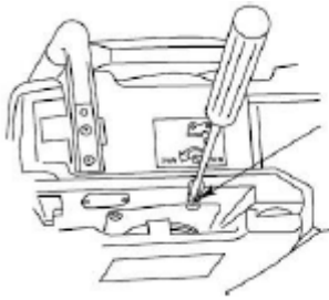
Chain oil flow adjusting
