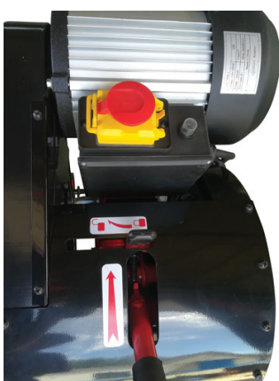
Close-up image of lever and emergency stop.
